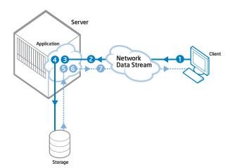
**Figure 1. Data paths to and from application.** Server overhead and response latency occurs throughout the request-response data path. These overheads and latencies include processing incoming request TCP/IP packets, routing packet payload data to the application, fetching stored information, and reprocessing responses into TCP/IP packets for routing back to the requesting client.
