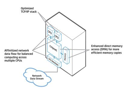
Figure 4. Intel<sup>®</sup> I/OAT performance enhancements. Intel<sup>®</sup> I/OAT implements server-wide performance enhancements in all three major server components to ensure that data gets to and from applications consistently faster and with greater reliability.
